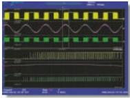
Measuring inverter I/O signals and control signals using the 10 MS/s high-speed 12-bit isolated module, current probe 700937 and isolated probe 700929
